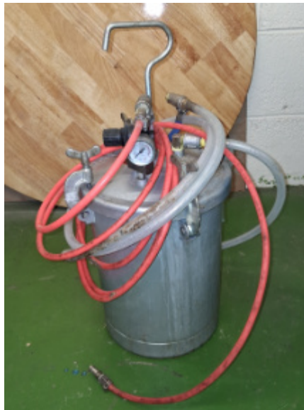
A paint pressure pot was used for injecting the resin into the floor
